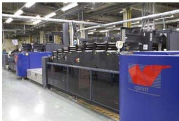
The latest addition to the VPrint technology is the first installation of its type in Europe. 16 nine inch (228.6mm) full-colour Kodak Versamark Printheads have been installed on a Matti transport system developed especially for this end application, producing full-colour reel-to-reel material on 2up duplex.
